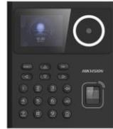
Face recognition terminal adopts deep learning algorithm, which helps to recognize the face faster with higher accuracy. It also supports multiple authentication modes: face/card/fingerprint/PIN authentication, etc. It can be applied in multiple scenarios, such as buildings, enterprises, financial industries, and other important areas.
